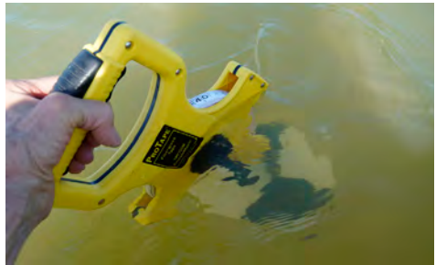
Above: Julie Youmans measures water clarity using a Secchi disk.
