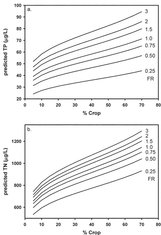
**Figure 5.**—Response of TP and TN to variation in %crop and flushing rate (FR) for reservoirs in the Missouri Plains as predicted by equations 5 and 11 in Table 2.
