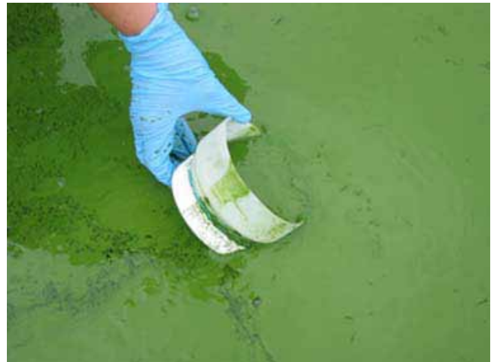
Above: A 64 µm net sampling a blue-green algae bloom at Binder Lake, Iowa.
