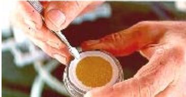
You will notice when you take the chlorophyll filter out of its filter house that the two sides look different: one has a regular pattern to it and is relatively smooth and one is bumpy and irregular. Place the smooth side down on the filter base with the rough side facing up toward you.
